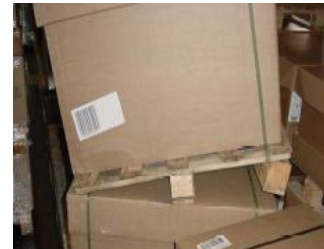
LACK OF DECKBOARD
